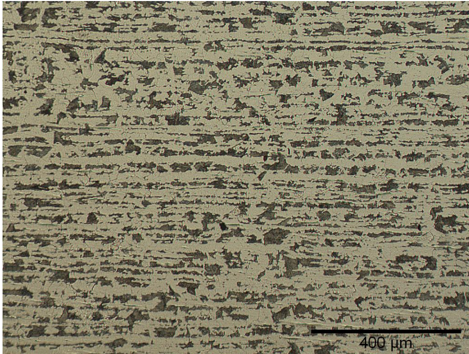
Figure B-3: Micrograph of Slow-cooled Plate A-3. 100 X.
