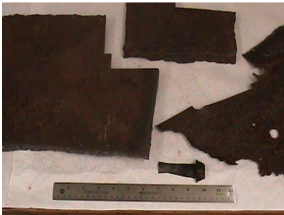
Figure 1: Photograph of selected steel pieces from the U.S.S. Arizona at Waipio Point. Left: Plate A-1. Top: Plate A-2. Right: Plate A-3. Bottom: Rivet.
